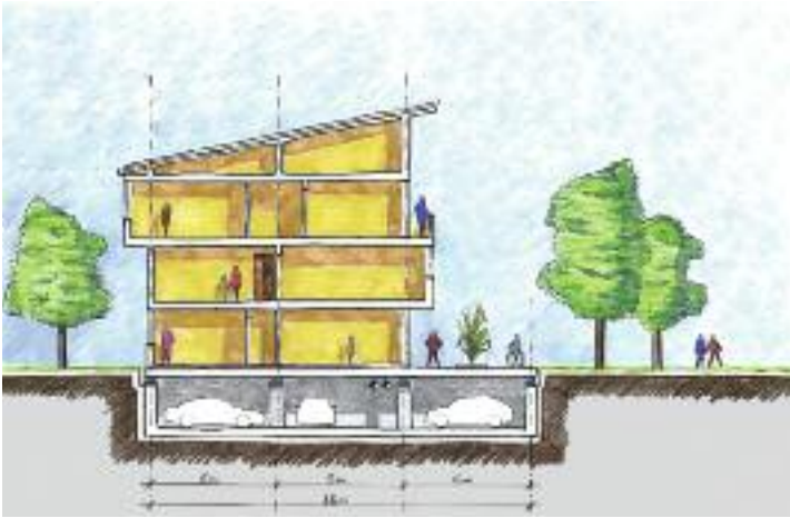
Fig. 1 One of the first sketches of the project illustrating the logic of the buildings constructed on isolated plates.
