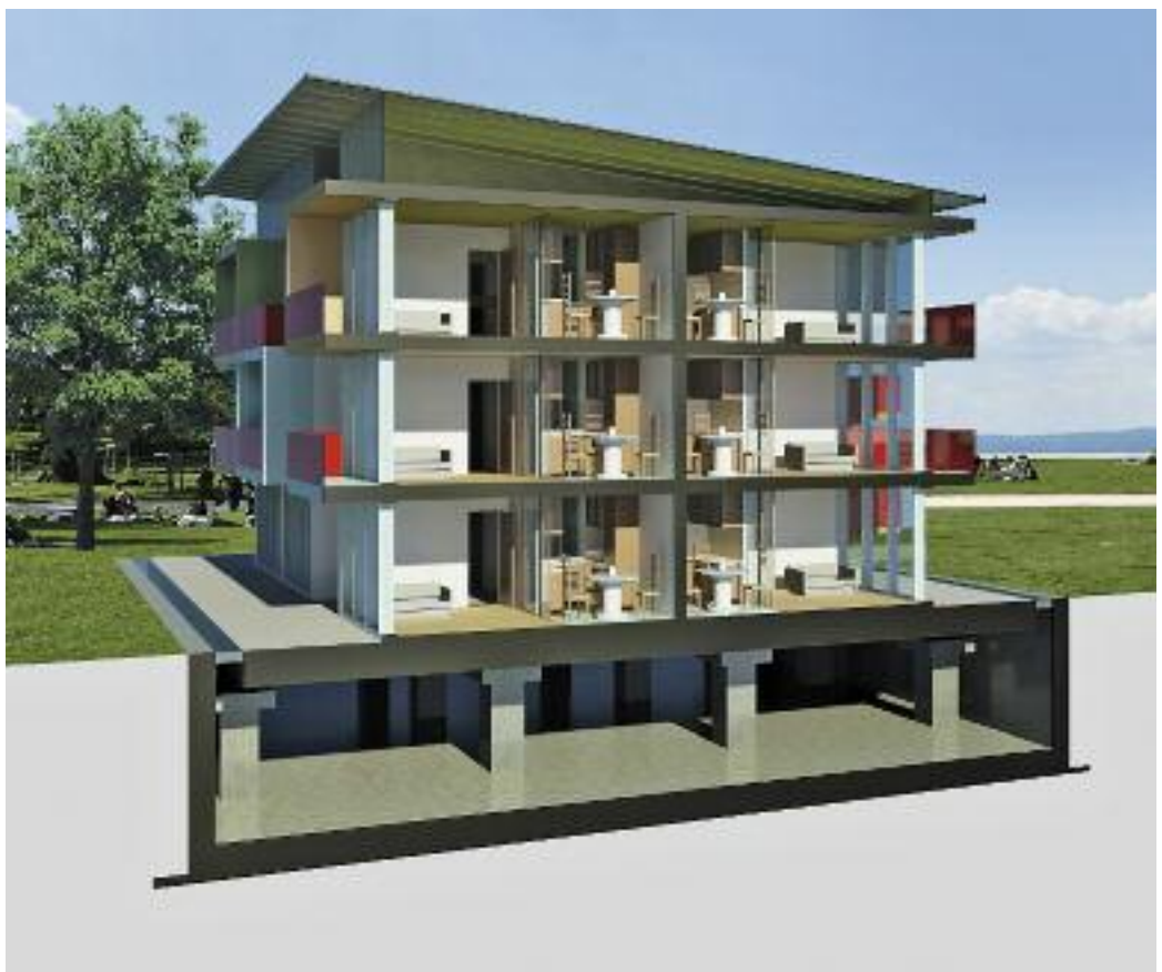
Fig. 1 One of the first sketches of the project illustrating the logic of the buildings constructed on isolated plates.
